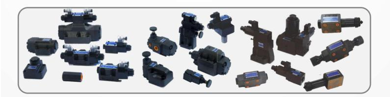
Solenoid Valve : DSG 01 to DSHG 10 i.e Flow From: upto 1100 LPM Pr 315 bar **Relief Valve** : BG, BSG, BT, SERIES Type flow: upto 650 LPM Pr: 350 bar : MPW, MSW, MRP, MBP SERIES Flow: upto 400 LPM Pr: 315 bar **Modular Valve** Electro Proportional Valve: EDG 01, EFBG 03 /04/06/10 Flow Control Upto 500 LPM Pr 245 bar
